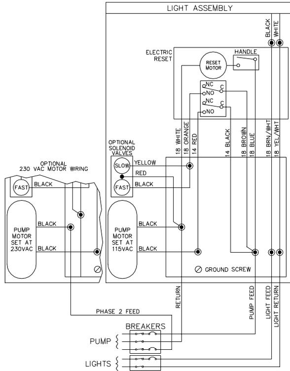
230 VAC WIRING (WARNING: ONLY FOR UNITS CONSTRUCTED SPECIFICALLY FOR 230VAC APPLICATIONS)
