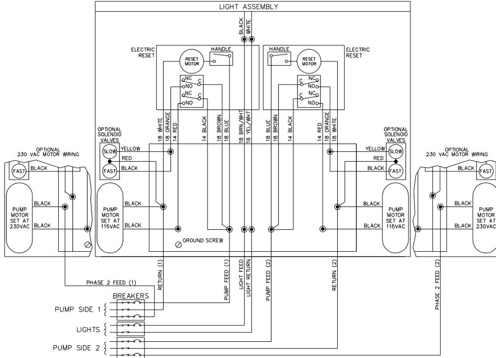
230 VAC WIRING (WARNING: ONLY FOR UNITS CONSTRUCTED SPECIFICALLY FOR 230VAC APPLICATIONS)
