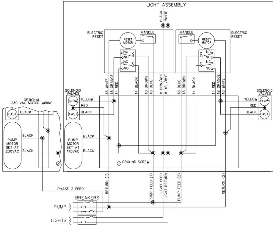
230 VAC WIRING (WARNING: ONLY FOR UNITS CONSTRUCTED SPECIFICALLY FOR 230VAC APPLICATIONS)
