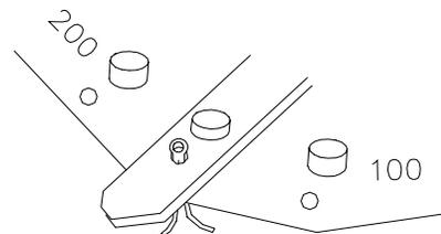
5. If you have difficulty reaching the dollar shift lever when changing prices, remove the two cap screws located over the tabs of the bezel assembly. Lift the bezel assembly upward and remove it from the unit. When reattaching the bezel to the dispensing unit, be sure the top inner edge of the bezel assembly slides into the U-shaped channel located on the upper edge of the dispensing unit.
