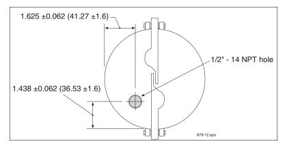
Figure 6. Modifying An Existing Metal Riser Cap
