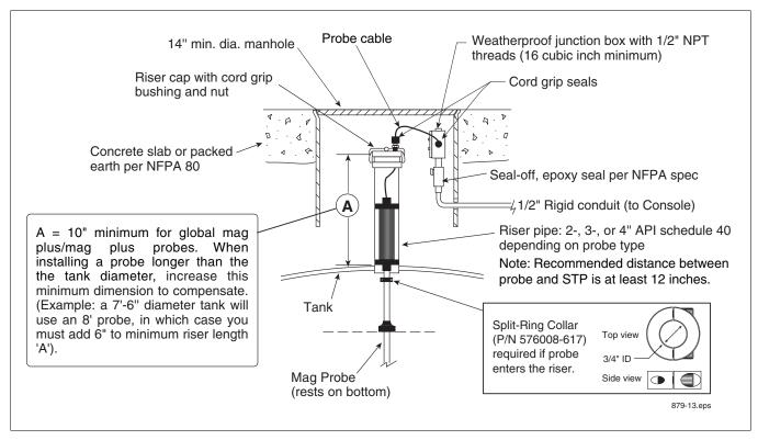
Figure 12. UST Mag Plus Probe Installation - Dedicated Riser
