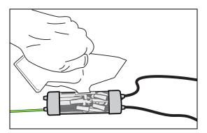
Figure 20. Pouring Sealing Compound Into Sleeve
