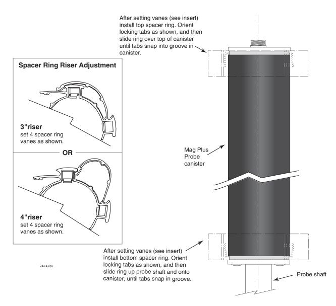
Figure 10. Installing Mag Plus Probe Canister Spacer Rings
