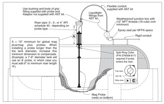
Figure 14. AST Mag Plus Probe Installation - Dedicated Riser
