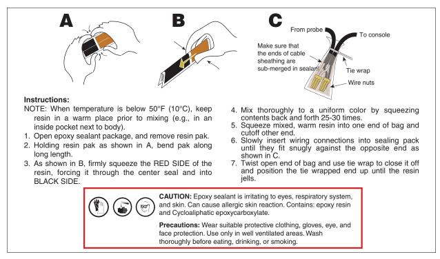
Figure 16. Epoxy Sealing Mag Plus Probe Field Connections
