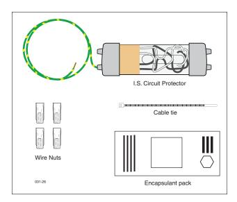
Figure 8. I.S. Circuit Protector Installation Kit Contents
