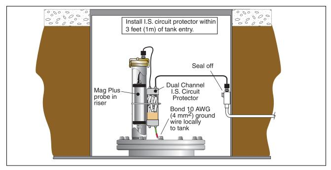
Figure 13. Optional UST Mag Plus Probe Installation With I.S. Circuit Protector
