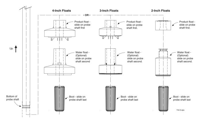
Figure 11. Mag Plus Probe Float Installation
