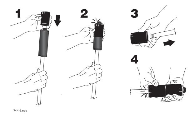
Figure 9. Installing Mag Plus Probe Canister Insulator Sleeves
