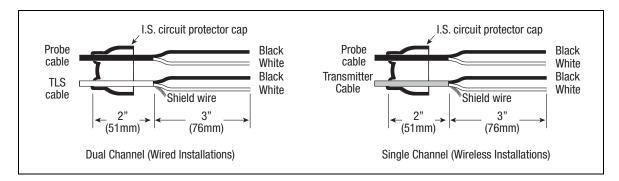
Figure 17. Splice Length Dimensions
