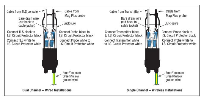
Figure 18. I.S. Circuit Protector Splice Connections
